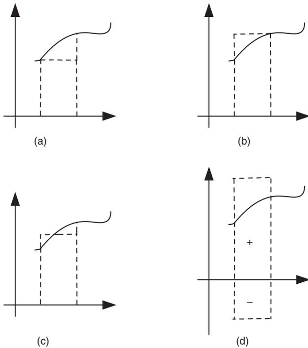
Figure 1. (a): Forward difference (Euler), (b): Backward difference, (c): Tustin's, (d): GBT with  $\alpha > 1$ .
