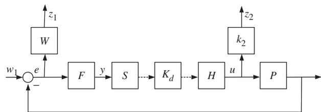
Figure 9. Sampled-data feedback system.
