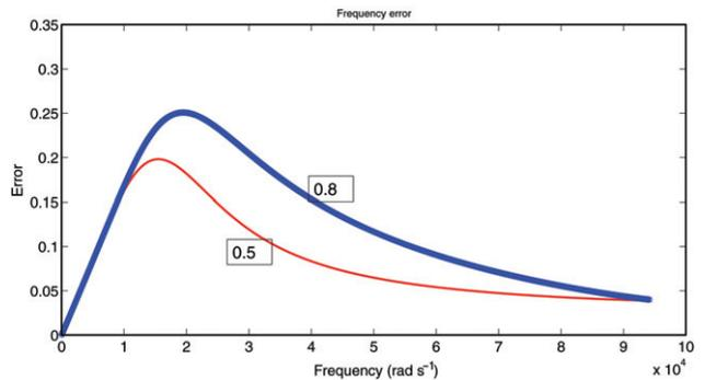
Figure 4. Errors in the frequency domain.
